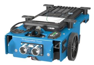
Rover is an introduction to coding and robotics. The simple programming language ( TI basic ) that is built into TI graphing technology makes it easy to program the system, run it and troubleshoot to correct or fine-tune performance.
