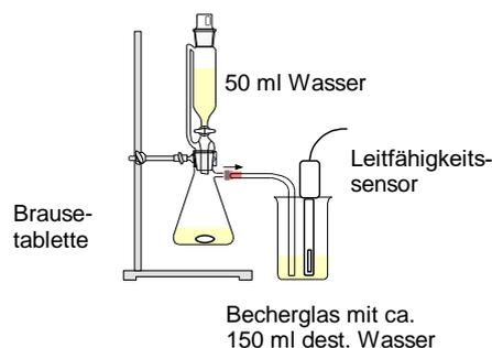
Prepare the computer with connected conductivity sensor (measuring range 200  $\mu\text{S}$ ) for data recording so that a measured value is recorded every 5 seconds for a period of 300 seconds.
