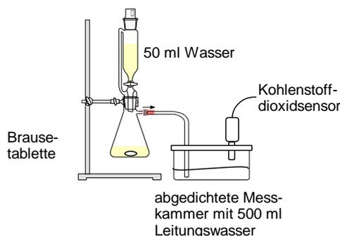
Prepare the computer with connected CO<sub>2</sub> sensor for data acquisition in such a way that a measurement value is recorded every 10 seconds for a period of 600 seconds. Start the data acquisition. After approx. 30 seconds, open the tap on the dropping funnel so that water is directed drop by drop to the effervescent tablet and carbon dioxide is slowly introduced into the water. Save the recorded data at the end of the measurement.
